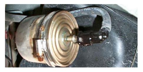
**6.** After the fuel has drained (takes some time) remove the other fitting At this point more fuel will leak out.
