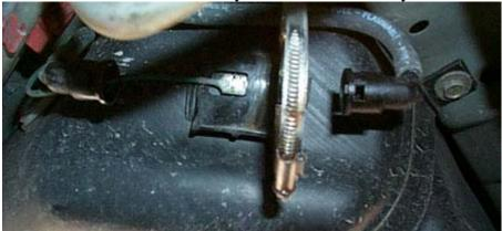
9. Now put the new filter in the loop and tighten the screw.
